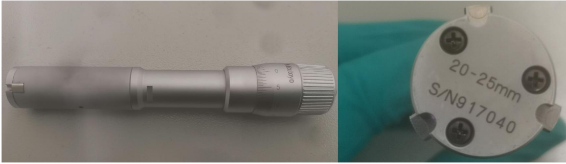
Figure 3.17: The micrometer for the inner radius measurement(left) and three anvils at the bottom(right)
