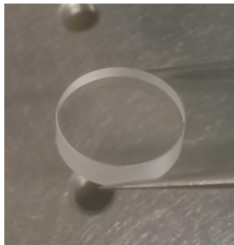
Figure 3.6: A photo of one of the sapphire samples
