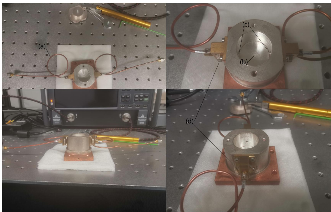
Figure 3.2: Real pictures for the resonator. (a) The cable ; (b) the PTFE rod used to fix the support at the bottom; (c) loops at the end of the cable to excite resonance modes; (d) the gear able to be rotated to adjust the distance between the loop and the symmetric axis of the resonator;
