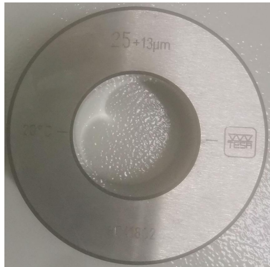
Figure 3.18: The set ring with a diameter 25 \text{ mm} + 13 \mu\text{m} at 293 \text{ K}
