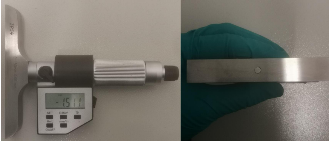
Figure 3.19: The depth micrometer(left) and the moving spindle at the bottom(right)
